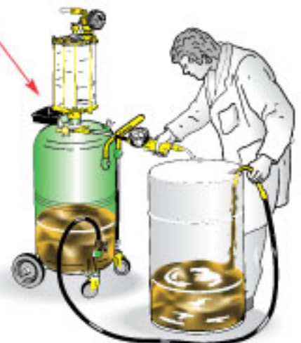
2 m hose for draining of tank with air.
