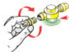
Unit with safety valve 1 bar and universal cock 1/4" G
