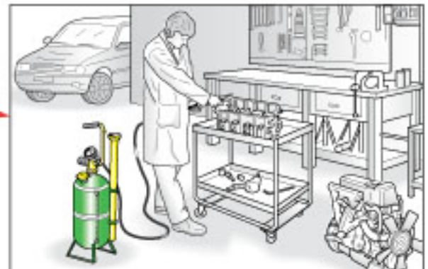
Draining small quantities of residual liquid when overhauling an engine.
