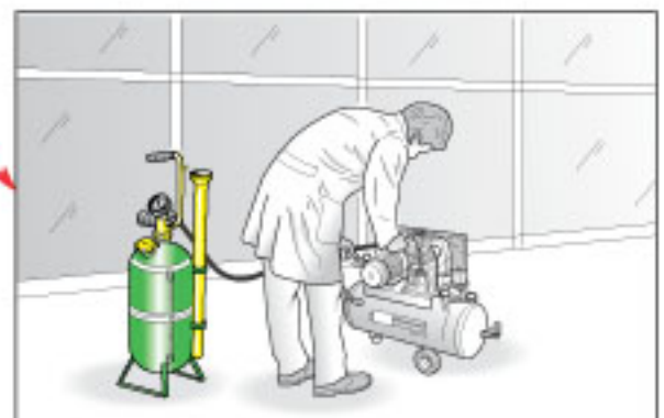
Draining for oil change in a small compressor for normal maintenance.
