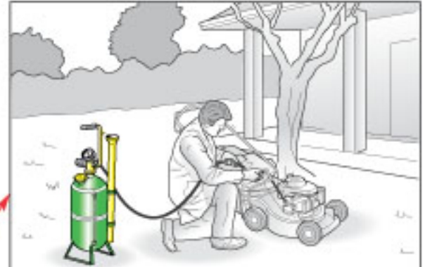
Draining of waste oil when servicing a lawnmower.
