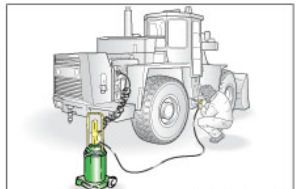
Proceed with maintenance by feeding the grease pump with air produced by the bulldozer
