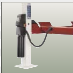
Pump and control units placed on front rear post.
