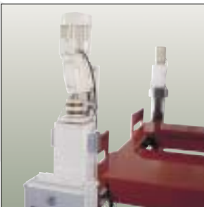
Gear motor and elastic coupling which ensure that load spindle/nut is always axial.
